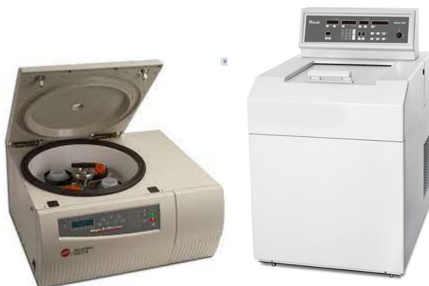
Fig. 3.3: Photographs of benchtop centrifuge and refrigerated high speed centrifuge.
