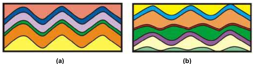
Fig. 10.23: a) Harmonic fold; and b) Disharmonic fold.
