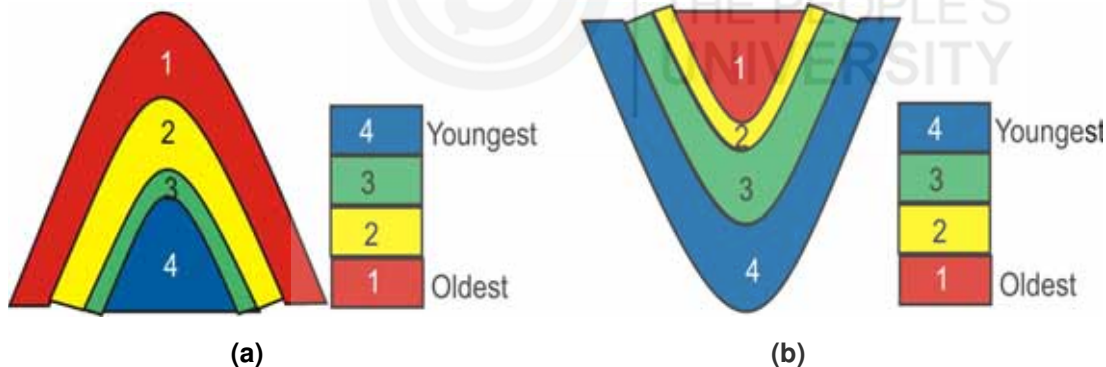
Fig. 10.9: a) Antiformal syncline; and b) Synformal anticline.
