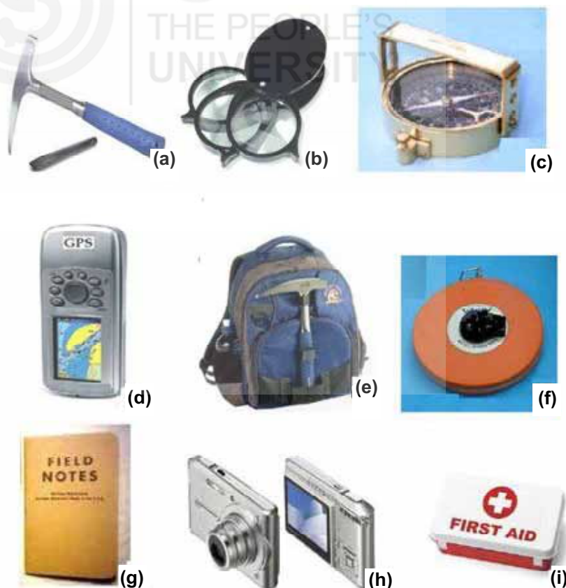
Fig. 13.4: Field equipment (a) hammer and chisel, (b) hand lens, (c) clinometer, (d) GPS, (e) haversack, (f) measuring tape, (g) field notebook, (h) digital camera, and (i) first aid box
