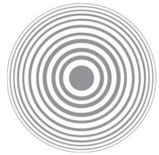
Fig. 8.4: Circular fringes observed in a Michelson interferometer.
