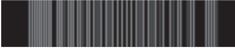
Fig. 6.10: Interference fringes produced in the Fresnel biprism experiment.
