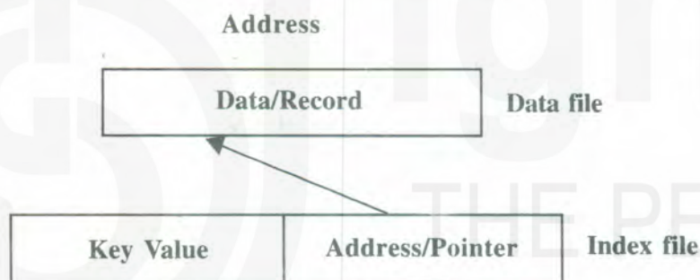
Fig. 2.8: Data Access Using Index File
