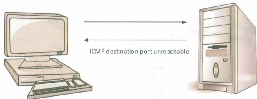
Fig. 16: UDP scan result when the port is closed.
