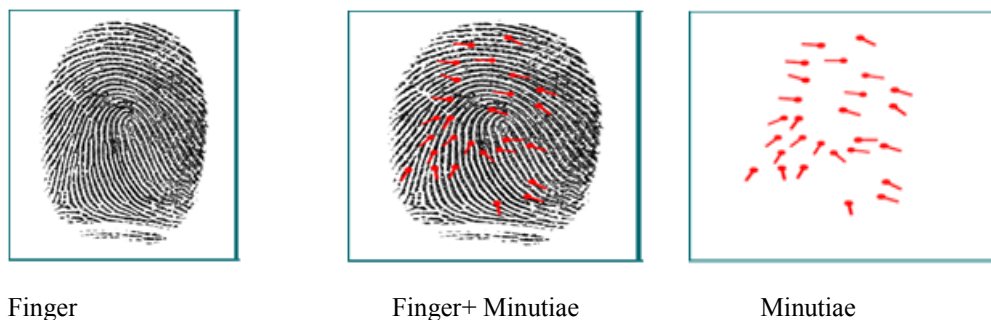
Figure 10: Extraction of Minutiae
