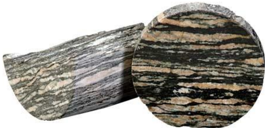
Fig. 14.20: Rock cutting polished surface showing schistosity or schistose structure. (Source : https://flexiblelearning.auckland.ac.nz/rocks_minerals/rocks/schist.html )
