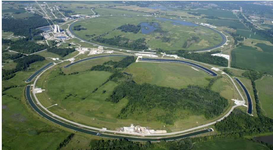
Fig. 3.2: Aerial view of the particle accelerator Tevatron at Fermilab, USA. Until 2007 it was the most powerful particle accelerator in the world, which accelerated protons to energies of over 1 TeV (tera electron volts = 10^{12} eV). Beams of circulating protons in two circular vacuum chambers in the two (6.28 km) rings shown in the picture collided at their intersection point.
